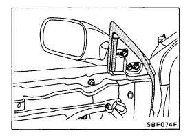
3. Tilt door mirror as much as possible in the direction shown below and tighten the 3 bolts.
