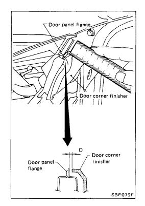
e. Apply butyl seal or equivalent around the 3 fixing clips or door corner finisher, and install it.
