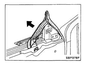
d. Bend door panel flange where door mirror is fixed so that the distance "D" between outer edge of door corner finisher and inner surface of flange is within specifications.
